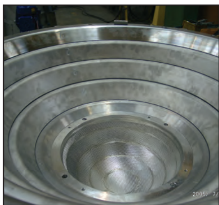
FIGURE 5. This photo shows the basket of a baffle ring centrifuge
