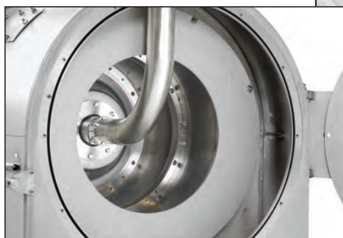
FIGURE 8. Closeups of the interior of two-stage (left) and three-stage (right) pusher centrifuges
